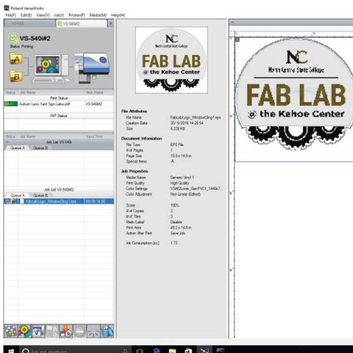
15. To make sure that our cut lines will actually cut, open the **settings** window. Navigate to the **Cut Controls** panel, and then make sure the **Operation Mode** is set to **Print & Cut**. You will have confirmation that your line will be cut when you see a line of red “**marching ants**” tracing your cut line. If you don’t see this, or you just see a magenta line, the machine will not cut the stickers.
