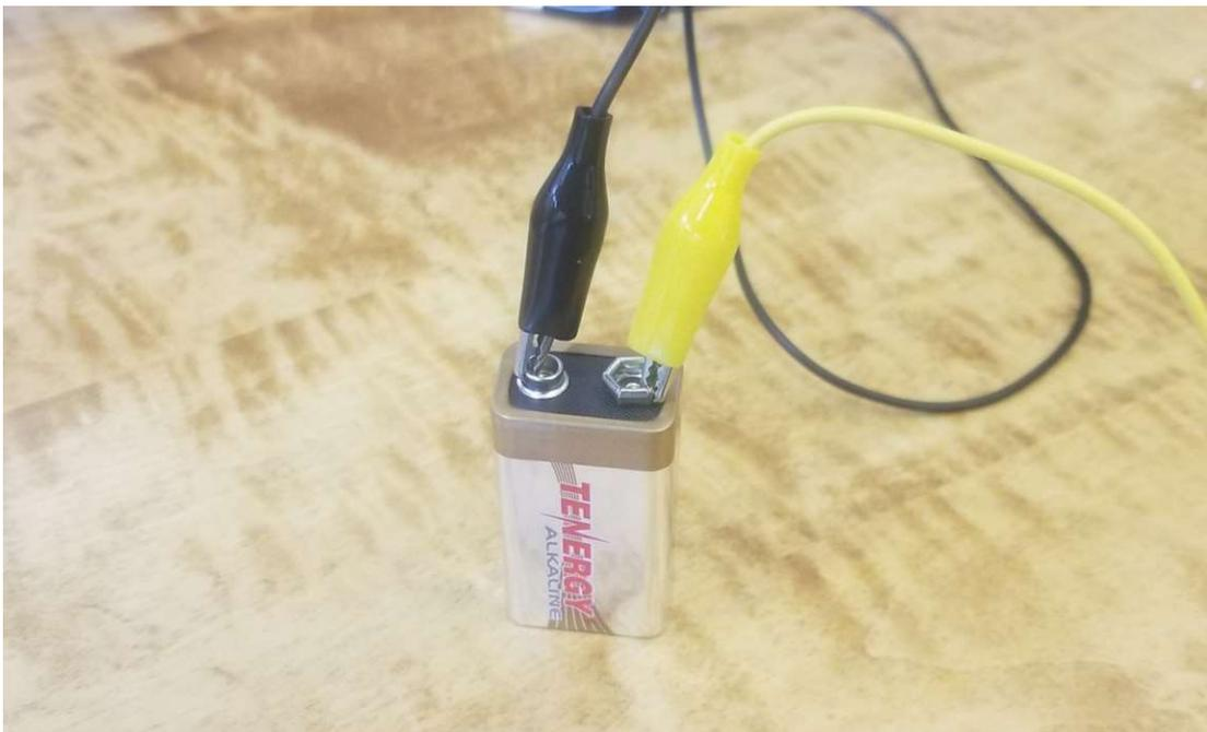
3. **Connect the other end of the clip attached to the battery's male pole to one of the terminals on the switch.** You will need to unscrew the plastic cover from the terminal to expose the metal bolt, but you don't need to fully remove it.
