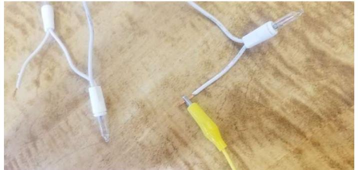
5. **Finally, connect a third alligator clip to the other end of the light string, and then attach it to the other silver terminal on the switch.**
