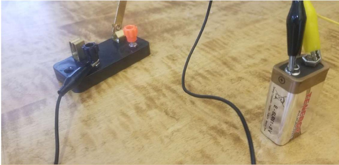
4. **Connect the other end of the alligator clip attached to the battery's female pole to one of the exposed copper wire ends of the light string.**
