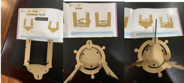
6. The locking plate needs to fit into the third pillar just like the other 2 pillars. Take 3 screws and put each one into a straw and then add a thin ring over each straw. Put each straw into each hole through the bottom disc. This is what it looks like with the three straws in the bottom disc.
