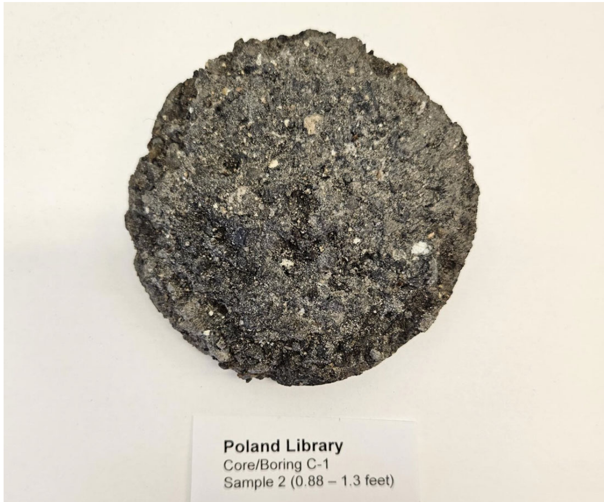
Fused slag obtained (cored) from C-1 (nominal diameter 4 inches). Note the presence of free lime within the specimen (white inclusions).
