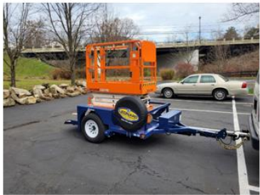
New Trailer (with existing scissor lift)
